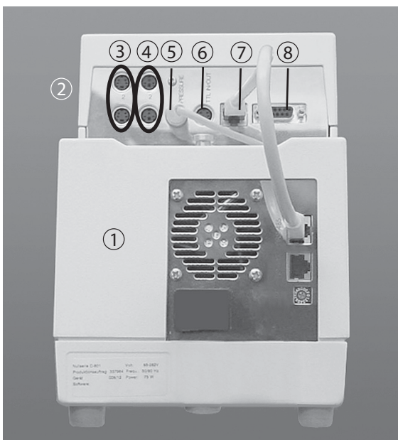
Fig. 5.10: Rear connections of the pump manager and the pump module
