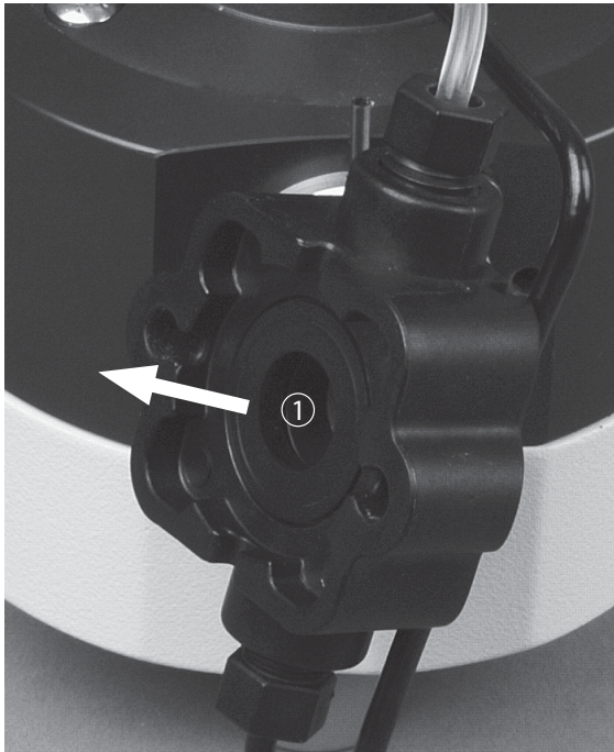
Fig. 7.1: Removing the radial seal
