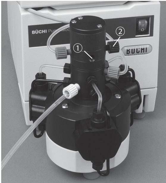
Fig. 5.13: Pump head with connected pressure tubing
