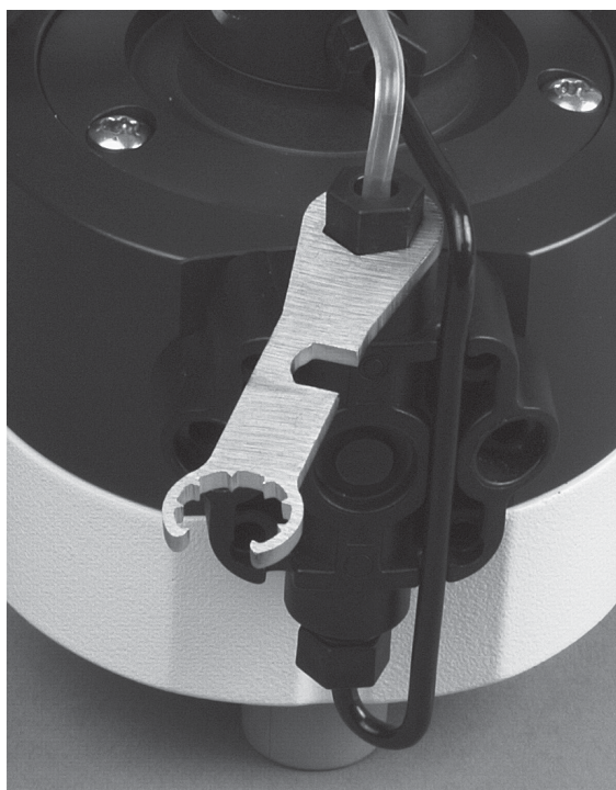
Fig. 7.4: Uninstalling the fitting
