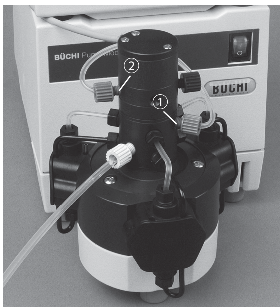
Fig. 5.12: Installing the suction tubing
