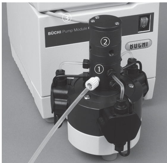
Fig. 5.11: Pump module with attached mixer
