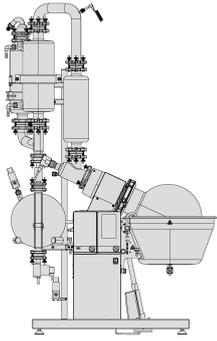
The R-220 Pro HP cont is the combination of the already well-known R-220 Pro HP and the R-220 Pro continuous. It offers the performance of the HP and the benefit of the continuous distillation.
