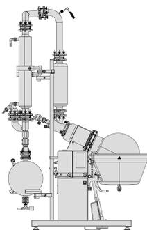
The glass configuration of the “High performance” version, consists of two parallel condensers to be able to condense the higher amount of evaporated solvent. Combined with two receiving flasks of 10 L each.
