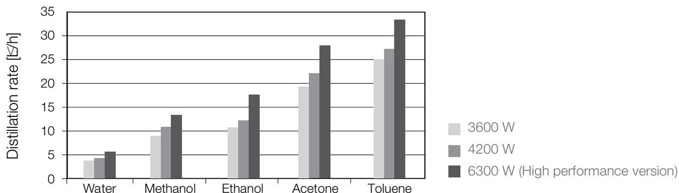
The maximum achievable distillation rate is not just related to the heating capacity, but also on rotation speed, flask size and temperature difference between bath and cooling.
