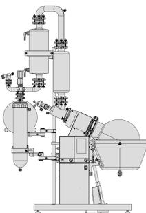
The R-220 Pro Extraction is based on the Standard R-220 Pro with a descending condenser, 1 receiving flask and the special 4 liter extraction chamber. It is designed for continuous cold extraction of natural products.
