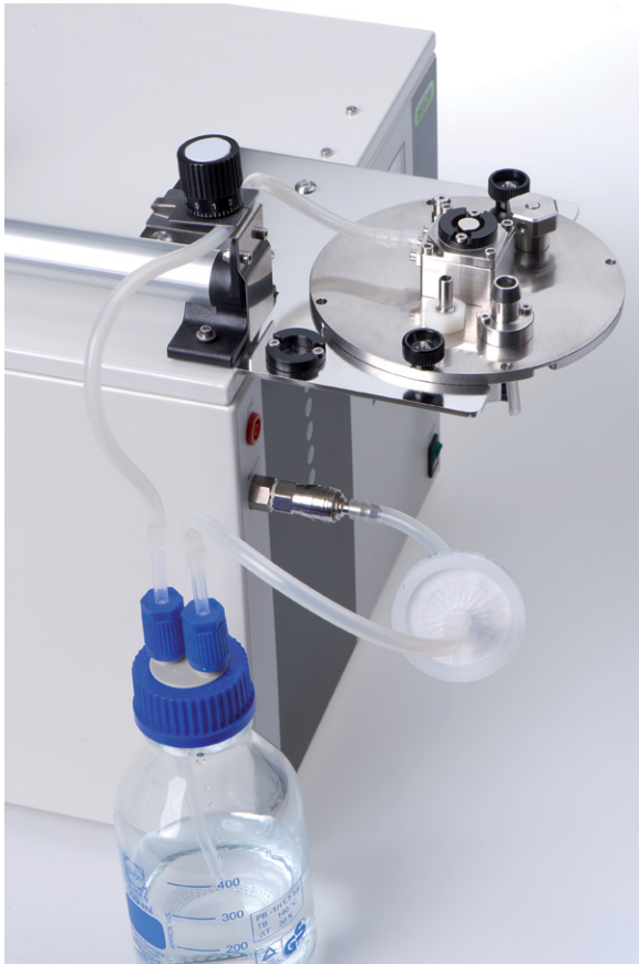
Figure 5-18: Installed pressure bottle
