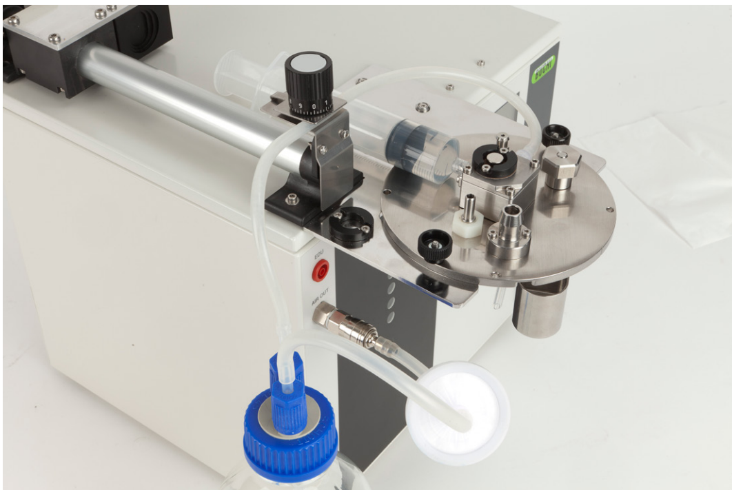
Figure 5-25: Installation of the CN system with one syringe pump and one pressure bottle
