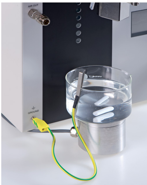
Figure 6-4: Grounding the open polymerization bath
