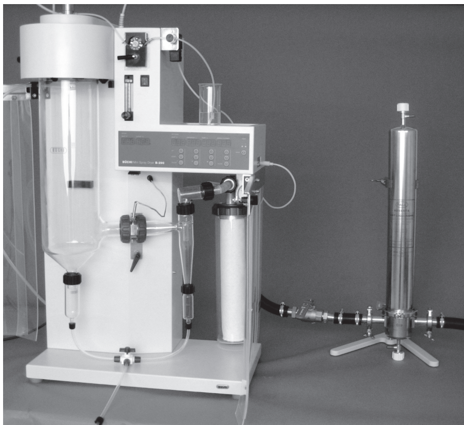
Fig. 5.11: Cleaning filter installed with stop cock
