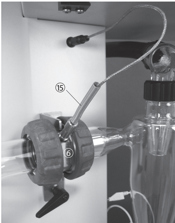
Fig. 5.2: Installing the glass assembly
