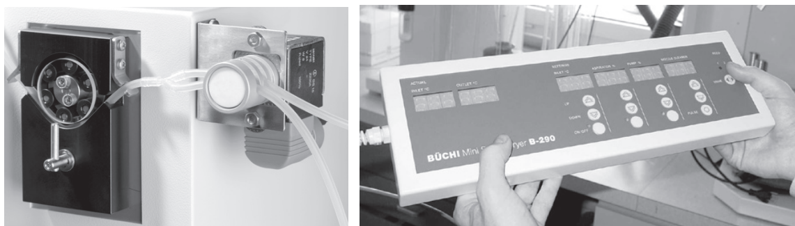
Fig. 4.7: Feed switch valve and remote control panel
