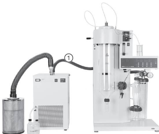
Fig. 5.23: Tubing between the Mini Spray Dryer B-290 and the Dehumidifier B-296
